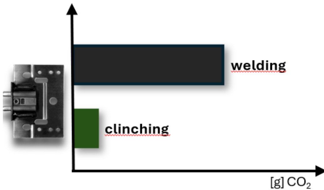
Figure 5 CO 2 emissions of welding versus clinching
