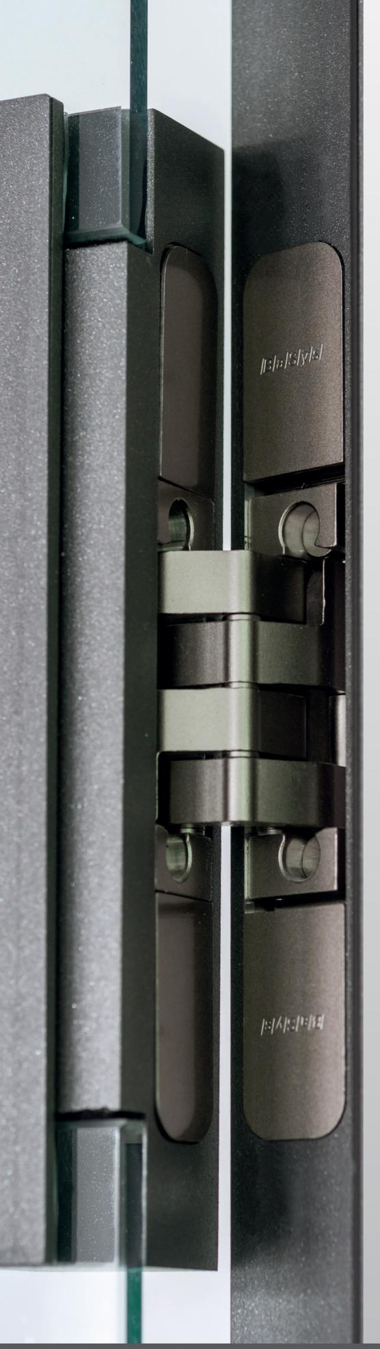
The frame part of the hinge disappears into the frame and the wing part vanishes into a retainer screwed into and therefore clamped to the glass door.
