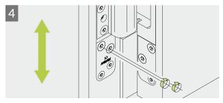
Height: slacken off the adjusting screws in the frame part. The hinge can now be moved 3 mm upwards or downwards. When the height is correct, tighten the adjusting screws slightly so that the teeth in the hinge engage.
