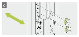
Joint clearance at the side: turn the adjusting spindles in the frame part of the **MASTERBAND** FX2 120 3-D CS to achieve exact positioning of the door leaf. The adjustment range is +/- 3 mm.
