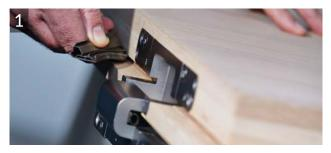
Once the hinge has been screwed into the wing, the wing seal is fitted. This is accommodated within the hinge with the aid of the sealing groove and continues in the joint area in the form of a seal specific to the hinge.
