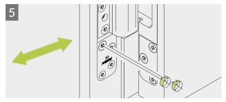
Seal contact pressure: push the hinge in the required direction (+/-1 mm); the teeth will hold the door leaf at the correct height. Fully tighten the adjusting screws in the frame part of the hinge.
