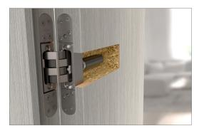
PIVOTA® DXS 101 3-D Close — the name refers to a concealed hinge that closes doors gently and automatically. The additional components not only adapt to the concealed system. The hinge also remains fully functional: it can be adjusted in three dimensions and enables the door to be opened to an angle of 180 degrees. In this state, the door remains open; the self-closing mechanism is only activated from an opening angle of approximately 110 degrees.
